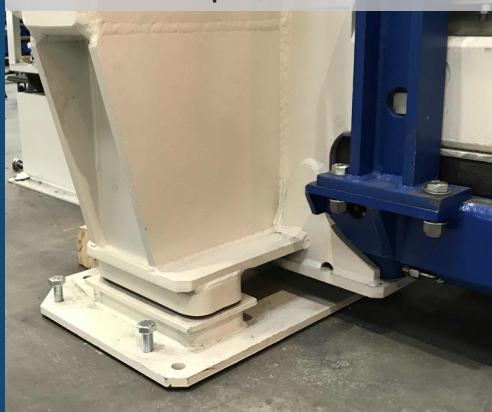
Elevated press frame based on anti-vibration suspension
